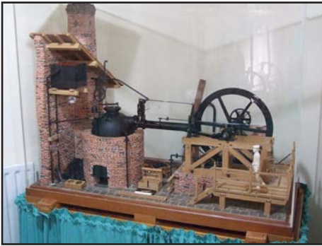
Richard Trevithick's high pressure engine 1804
