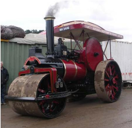
The roller, based at the Westbridge Depot, was used by the Highways Department for carrying out repairs to, and making new, roads until it was taken out of service during the 1960s. It was fitted with a scarifier at the rear on the right hand side to break-up the road surface prior to it being repaired. Although the Council bought a second roller (No 2), it never performed as well as No 1 and was eventually disposed of.
