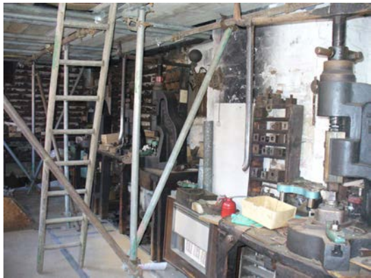
Evans Silver Factory - Fly press room with crash decking ©Steve Miles 2009
