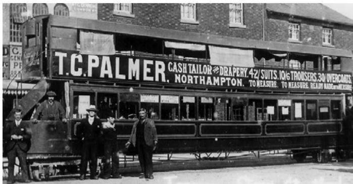
Here is one of the three huge 44 feet long, 100-seater, carriages of the Wolverton & Stony Stratford Tramway, built in 1887 by the Midland Railway-Carriage & Wagon Co Ltd of Shrewsbury. Note particularly the rudimentary protection for passengers seated on the top deck!
