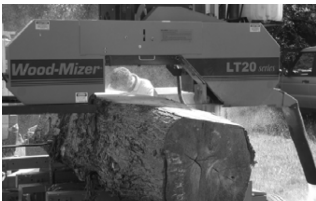
The 'table' being cut from a large piece of timber.
