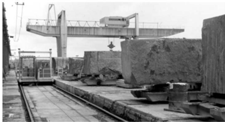
Rail Transferer for transfer of blocks from Quarry to stone saws in sheds on left. Carrières des Hainault Soignes
