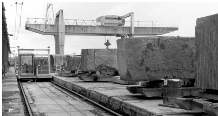
Rail Transferer for transfer of blocks from Quarry to stone saws in sheds on left
