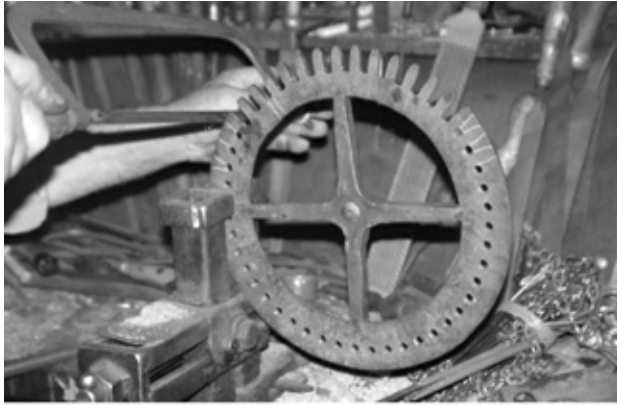
Martin Rowley cutting teeth in blank for Clock gear. Aug.2004
